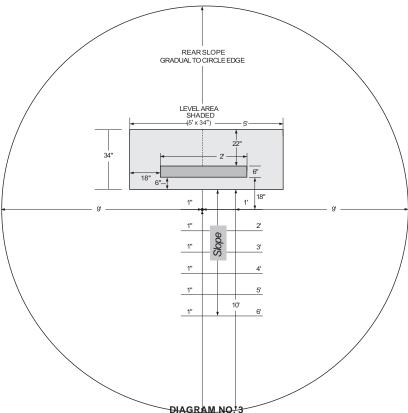
**Pitching Mound:** An 18' diameter circle, center of which is 59' from back of home plate.
